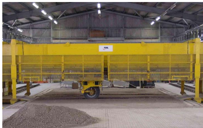
Figure 1, Full scale trafficking tests at the TRL Pavement Test Facility
